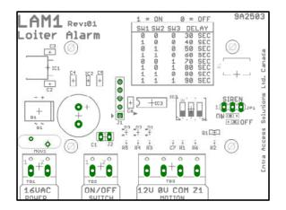
The Lam1 is a Local Loiter Alarm System. Its primary purpose is to prevent people from Loitering in enclosed areas, such as the bottom or top of stairwells, alcoves, and other such areas.)
