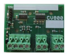
The CV800–SES series of Serial to Wiegand Converters is designed to interface to the SES™ TEC & CAT Telephone Entry Systems
