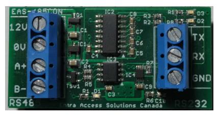
The EAS-485CON is an RS232 to RS485 Converter, It has Auto Baud detection between 9600 & 115200 Baud. It is a Plug and Play **device**, There are no User Settings
