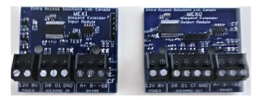
The WEX-KIT is a universal Wiegand extender (max64 bits). It consists of two(2) modules, the <u>WEXi</u> (wiegand input module) and the <u>WEXo</u> (wiegand output module). These Modules are designed to extend the standard Wiegand cable distance maximum up to 4000 ft(1200m) usig proprietary RS485 Communication between them.
