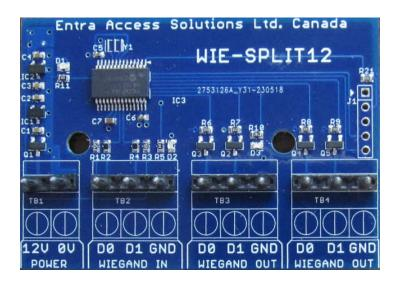
The WIE-SPLIT12 is an unisolated Wiegand Splitter, that takes Wiegand data from any Wiegand device (Max 64Bits), and outputs this identical data on the Two WIE-SPLIT12 output Ports .( The two Output ports are isolated from each other so there no feed back when connected in parallel to Card Readers.
