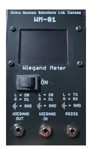
Entra Access Solutions Ltd, Introduces the first WM-01 Wiegand Meter/Analyzer. The WM-01 Wiegand Meter/Analyzer provides technicians with all the tools required to troubleshoot and Analyze Wiegand signals when Integrating Access Control Systems with Intercoms and Elevator control.
